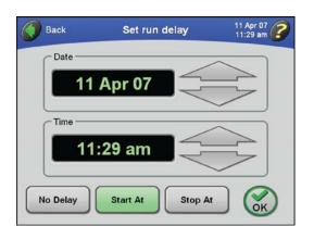
**a.** To set a delayed run to stop on a particular date and/or time, press the **STOP AT** button.
