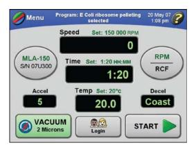
• The run parameters for the first step appear above the display fields in the Main screen.
