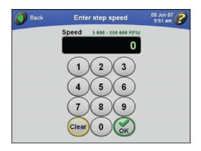
• The acceptable values for run speed are shown above the display field: from 5000 to 150,000 RPM, depending on the selected rotor.
