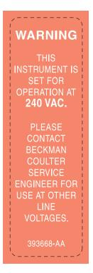
This symbol indicates that the instrument has been configured for operation at 240 VAC. Consult with a Beckman Coulter service engineer for use at other line voltages.
